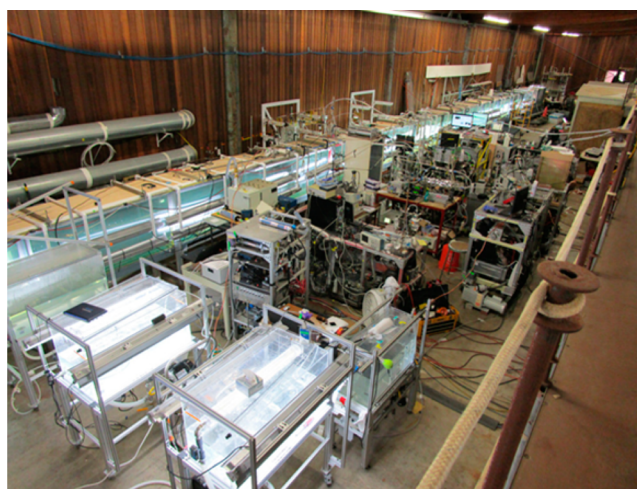
Figure 1. The 3,400 gallon wave machine in which the studies were completed. Image credit: the American Chemical Society. Reprinted from ref 1a.
